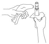
Figure U Lubricate Carb Tube
